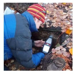
Figure 39. Measuring Electrical Resistivity and pXRF of KdVo-6 Sediments.
