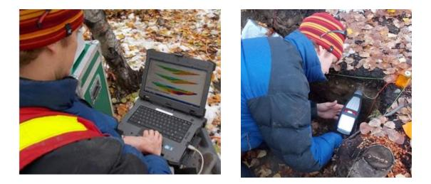
Figure 38. Measuring Electrical Resistivity and pXRF of KdVo-6 Sediments.
